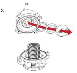
Make sure any unwanted spacers are removed from the top canister before making an adjustment to your spring rate.
