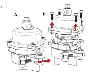
Caution! The cap of the BOV is under spring pressure. Be sure to secure the cap by press, vice, or clamp before removing the screws. Unscrew the 4x bolts with a 5/64" allen key.
