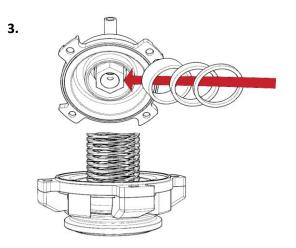
By using a combination of 0-3 of the spacers included, you will set your spring rate to work with the vacuum produced by your engine.
